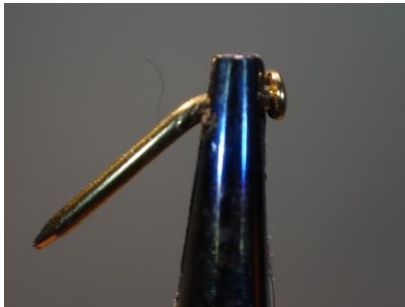
1 Bend the nail with fine point pliers
