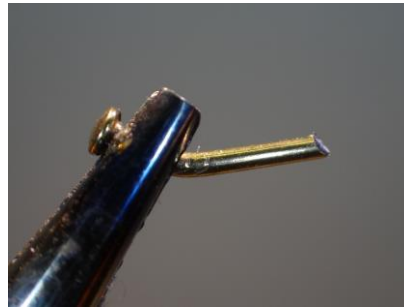
2 Cut off the point of the nail with diagonal pliers
